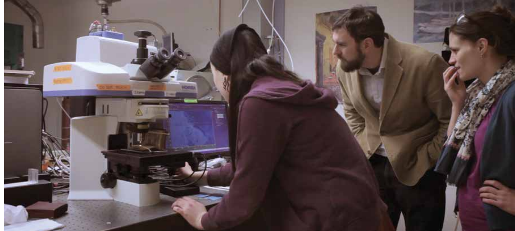
ABOVE: Chemistry major and art history minor Caren Sullivan '16, left, uses a confocal Raman microscope to determine which pigments are present in a 15th-century manuscript, while Assistant Professor of Art History Benjamin C. Tilghman '99 and Assistant Professor of Chemistry Allison M. M. Freshman look on. The work is part of Sullivan’s Senior Experience project.
