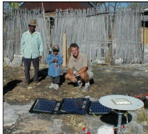
*Chuck DeMets uses GPS measurements to track tectonic plate movement in places like Mexico (shown here).*
